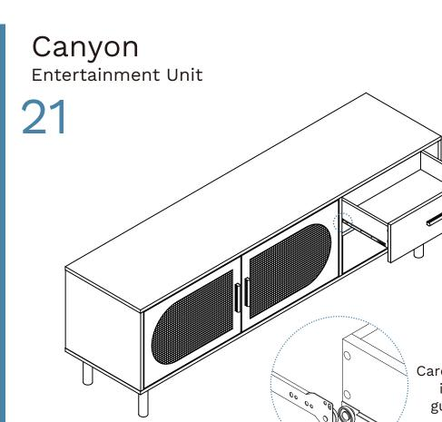
Carefully insert the drawers into the unit by gently guiding the runners into the tracks.
