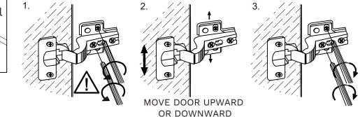
Unscrew 2 screws in round holes loosen 2 screws in oval holes a bit. Tighten 2 screws in oval holes. Screw in 2 screws in round holes
