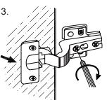
MOVE DOOR OUTWARD by turning this screw clockwise
